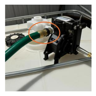
7. To adjust the proportioning ratio, loosen the black cap and turn the brass dial to set the desired concentration level. Begin at full strength (20%) and reduce gradually to around 10% if satisfactory results are achieved.
