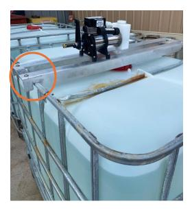
2. Make sure the white suction head is aligned directly over the red opening cap, as illustrated in image below.
