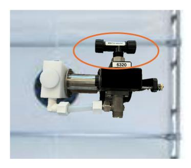
5. Connect the hose from the tap water to the filter on the proportioner as show below. Apply Teflon tape and tighten the connection. The hose connection is a regular 3/4-inch GHT (Garden Hose Thread).
